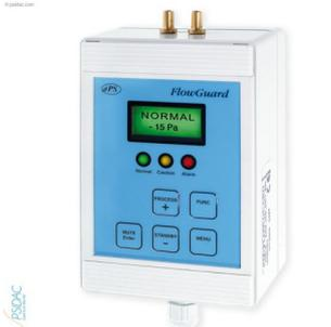
The FlowGuard 5290 is a high quality digital processor controlled flow and pressure monitor. Setup is very easy with the help of display and keypad. All parameters like alarm levels, alarm delays, unit, area, k-factor etc. can easily be modified to suite the application. The ceramic membrane and the capacitive technique used result in high accuracy and excellent long-term stability.
