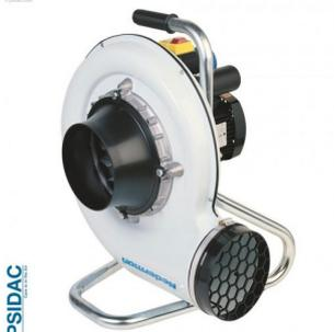
With LIFA 1600 you can easily perform leakage tests in ducts, buildings, filter banks etc. After the measuring object has been thoroughly sealed, an overpressure is created with the damper-controlled fan. The pressure difference over the supplied measuring tubes, with the help of the measuring tube diagrams, produces leakage air.
