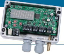
The FlowGuard 6283 v2 is an updated version with a faster and better processor with higher resolution. It's aimed for the advanced pressure, flow & airchanges measurement tasks. It's designed with the user and installer in mind. The 6283 v2 provide as much flexibility as possible in one transmitter.
